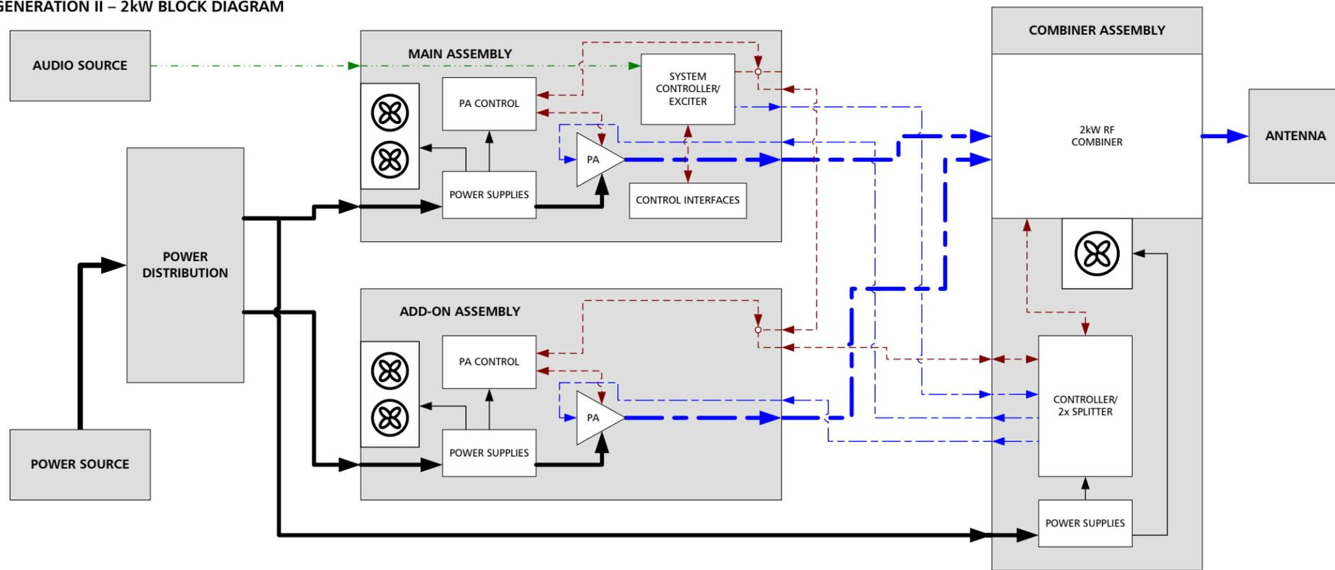
Figure 11 - STX LP Gen II 1kW and 2kW Block Diagrams
