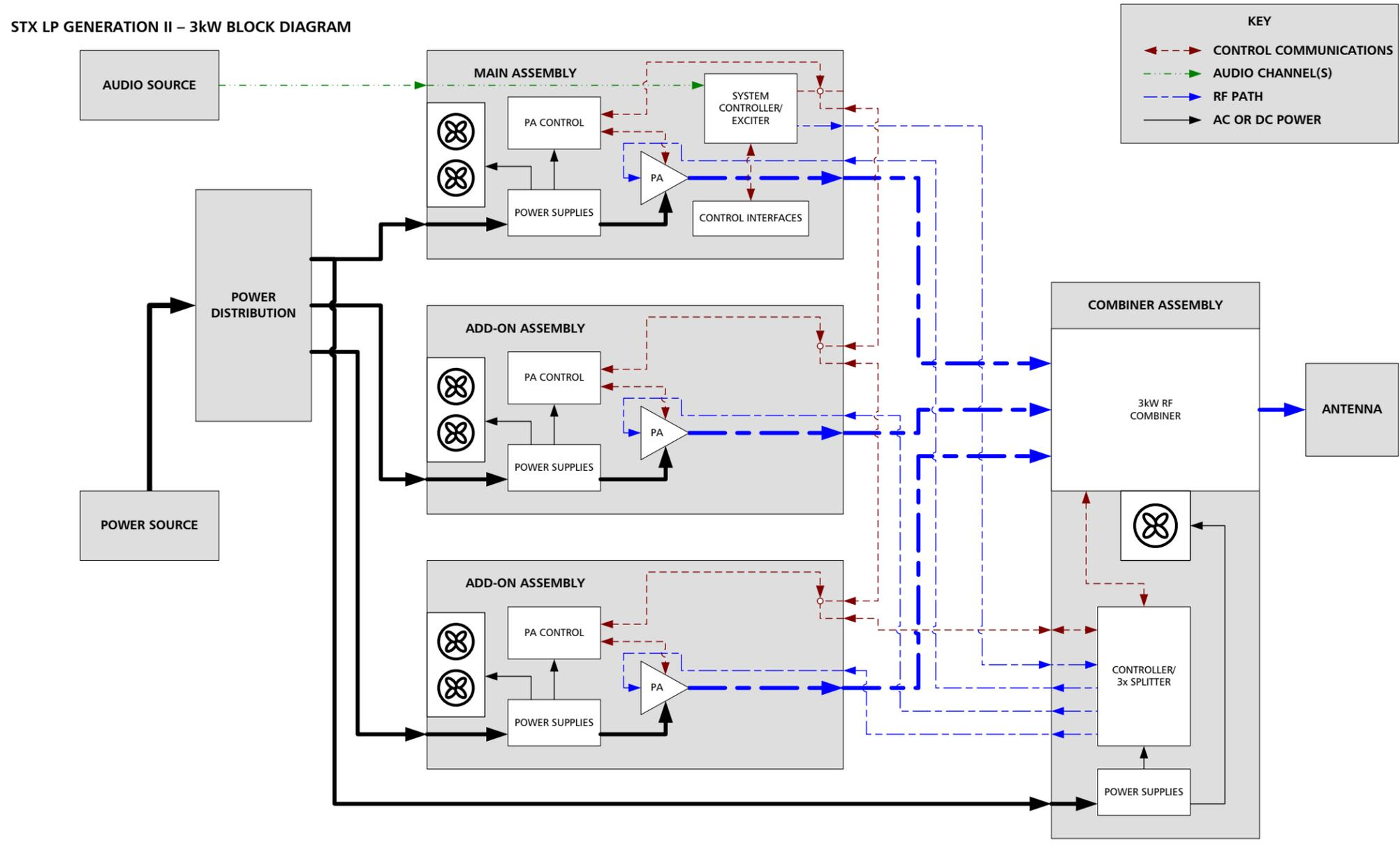
Figure 12 - STX LP Gen II 3kW Block Diagram
