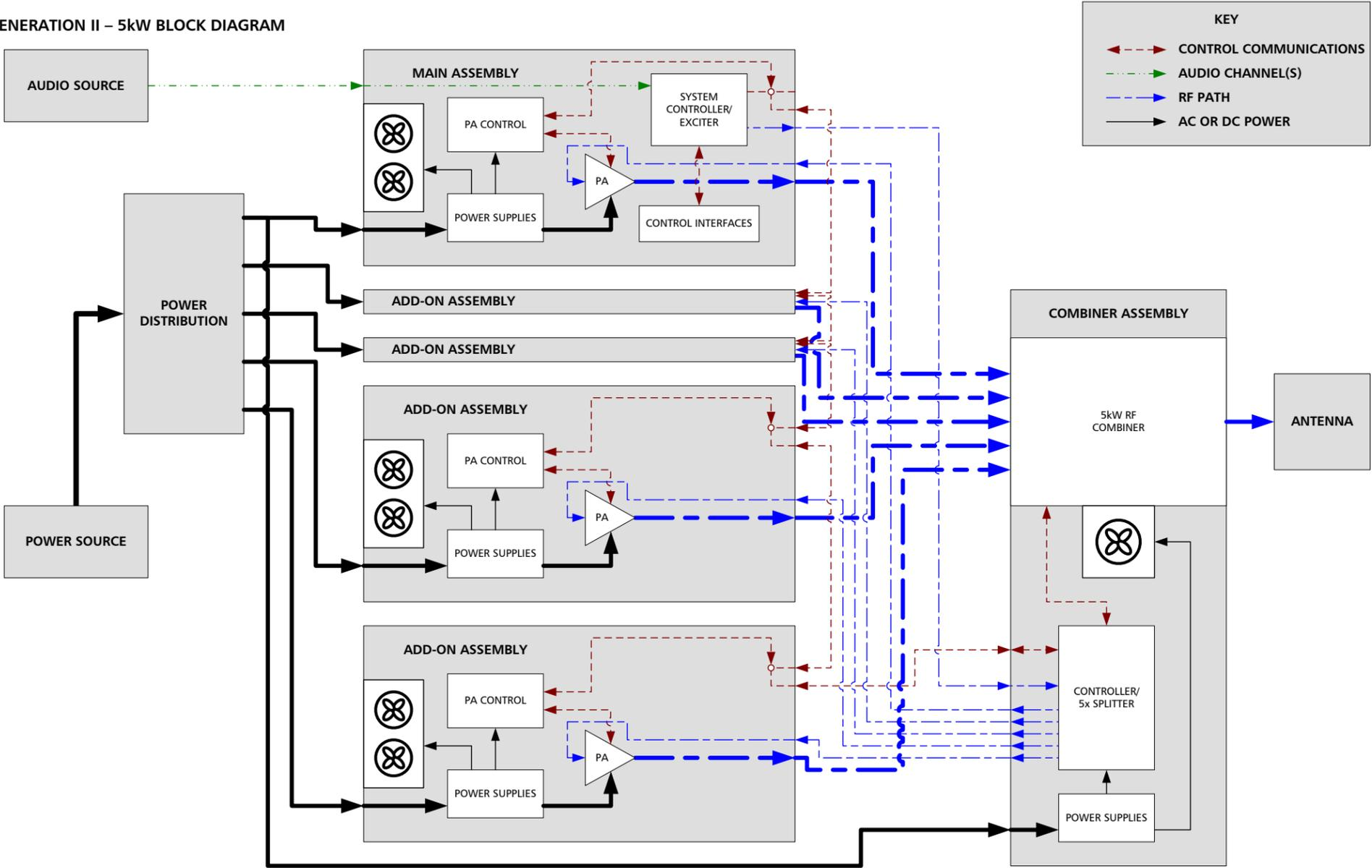
Figure 13 - STX LP Gen II 5kW Block Diagram
