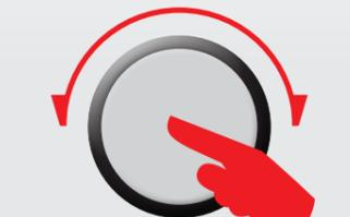
Turn the encoder to scroll through the menu and press to enter the selected item. Push the encoder a long time (more than a second) to return to the main screen.
