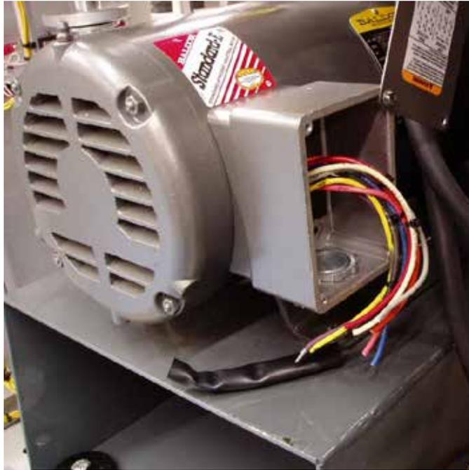
Figure 10 – Disconnect Harness from Blower Motor
