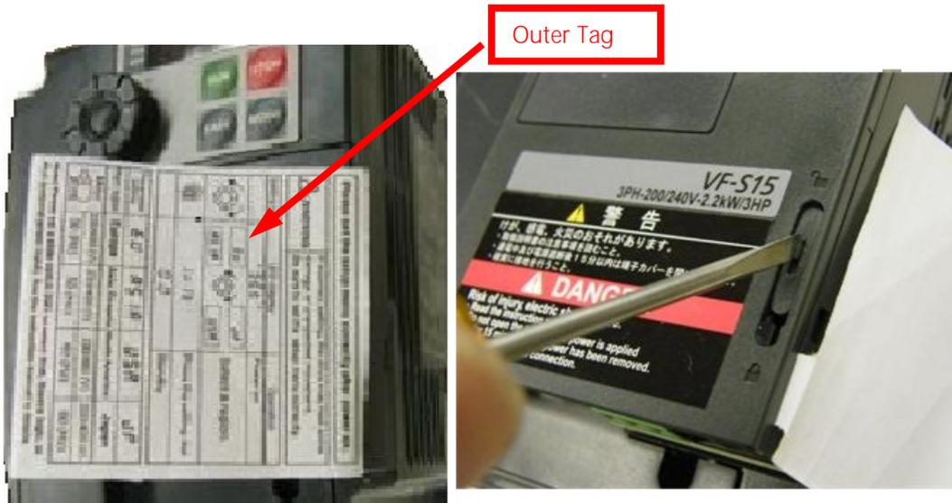
Figure 4 – Open Cover and Remove Outer Tag
