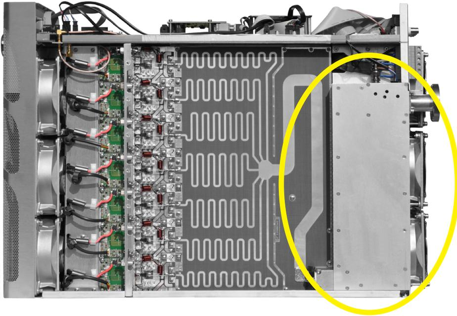
The low-pass filter is attached to the side walls:
