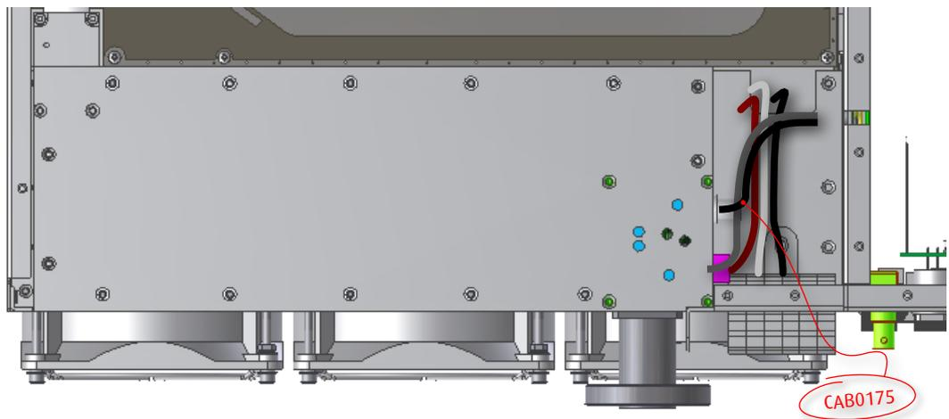
Given this mounting configuration, before work backwards to remove the filter, and then replace the new filter (that the Manufacturer sends you already tuned), restore all connections, close the transmitter and reconnect the power .
