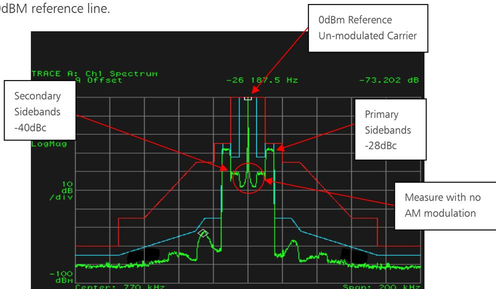
Figure 3 - 0dBm reference (Aligned AM IBOC Transmitter)
