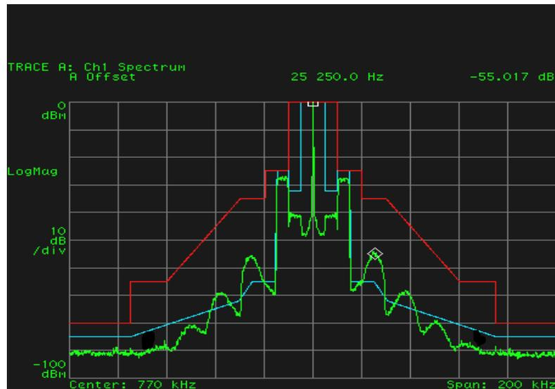
Figure 4 - Misaligned AM Transmitter
