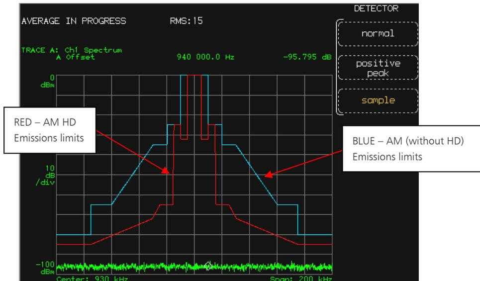
Figure 2 - Emissions Limits in Graphical Form
