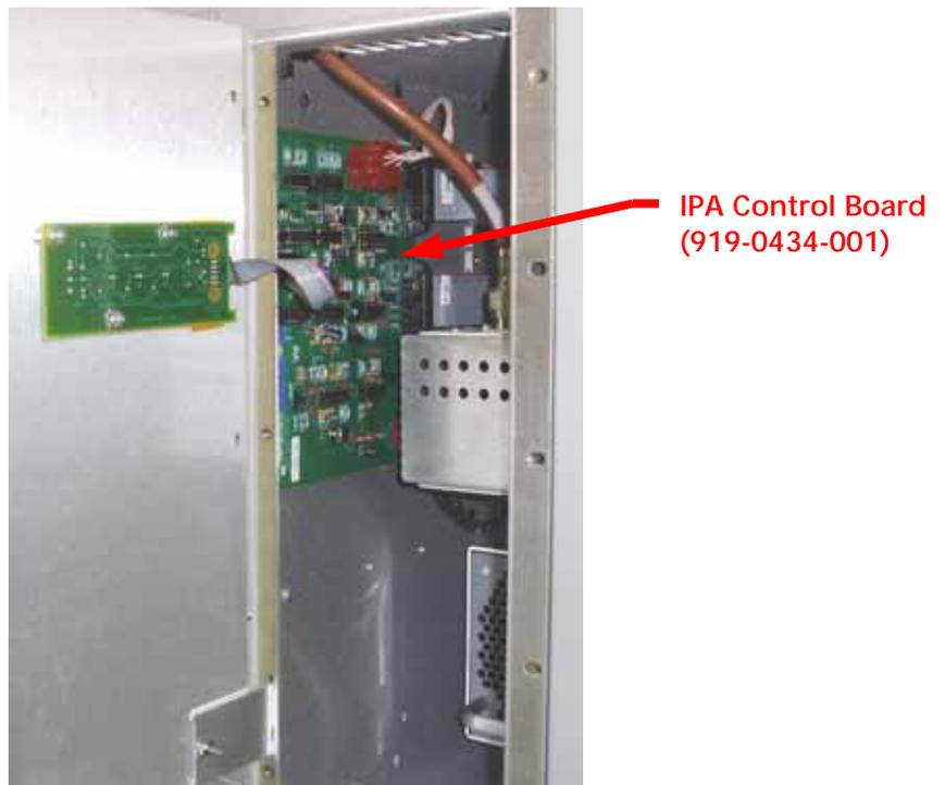
Figure 11 – IPA Control Board (919-0434-001) Removal
