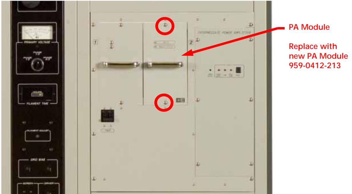
Figure 17 – PA Module (959-0412-213) Installation
