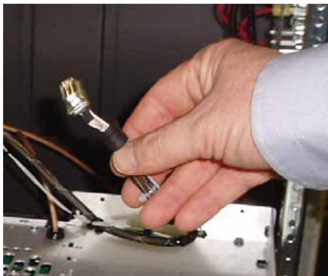
Figure 40 – Locate Exciter J3 Cable
