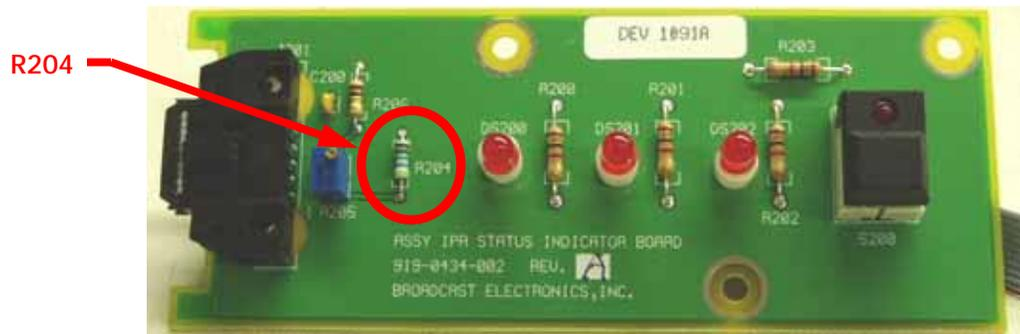
Figure 15 – IPA Status Indicator Board (919-0434-002) R204 Replacement
