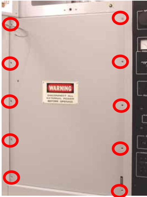
Figure 9 – Grid Compartment Cover Panel
