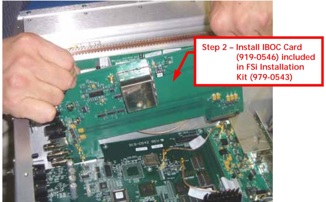
Figure 30 - IBOC Card Installation
