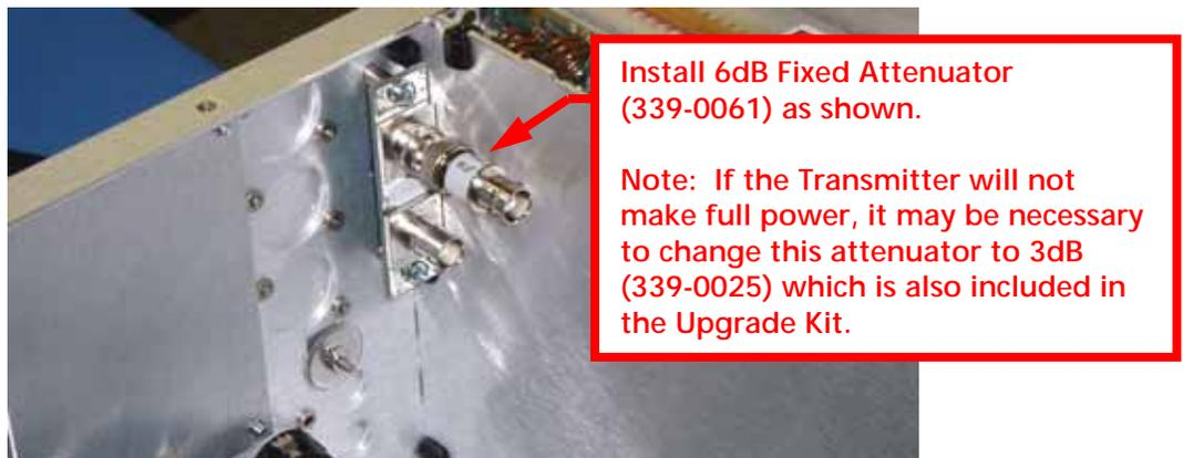
Figure 20 – Fixed Attenuator Installation
