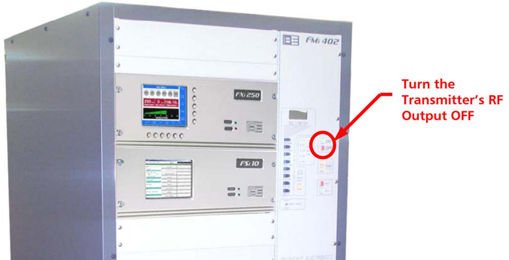
**Figure 1** – Turn the Transmitter's RF Output OFF
