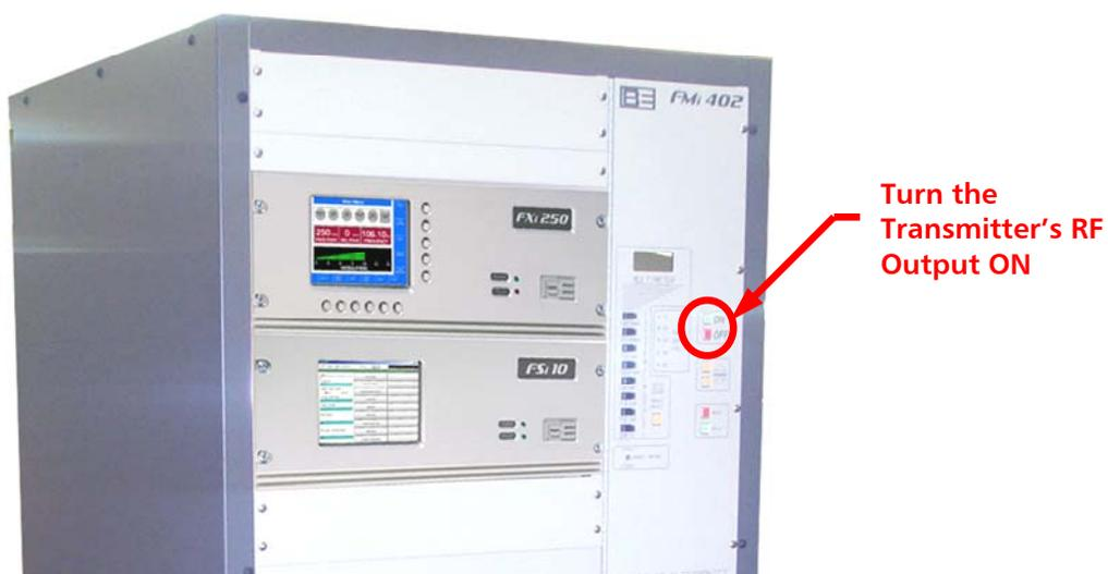
**Figure 15 – Turn the Transmitter's RF Output ON**
