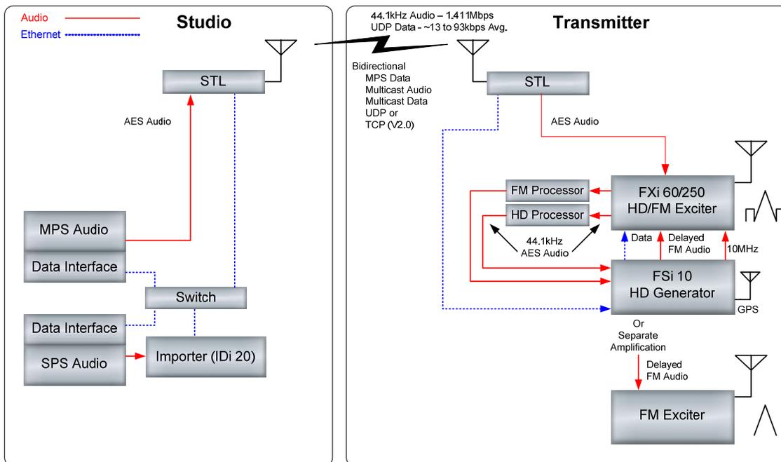
– Fig. 2: Multicast Architecture, HD Generation at Transmitter Site –
