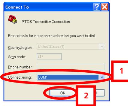
**Figure 15 – HyperTerminal Connect To Menu**
