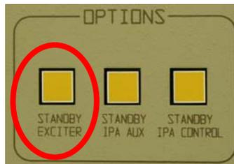
**Figure 23 – Standby Exciter Switch**
