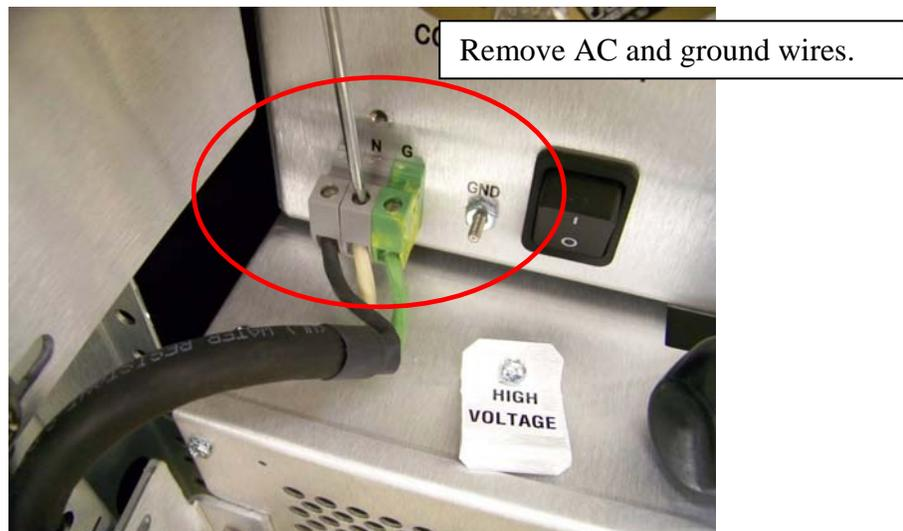
Figure 2. Remove wiring
