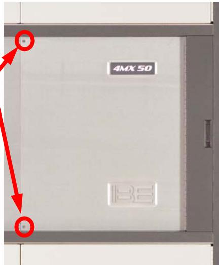
**Step 2** – Using a No. 2 Phillips Screw Driver remove the (3) screws from the hinge area as shown
