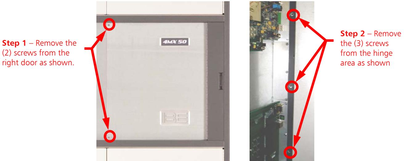
Figure 86 – Remote Control I/O and Audio Input Access Panel Hardware
