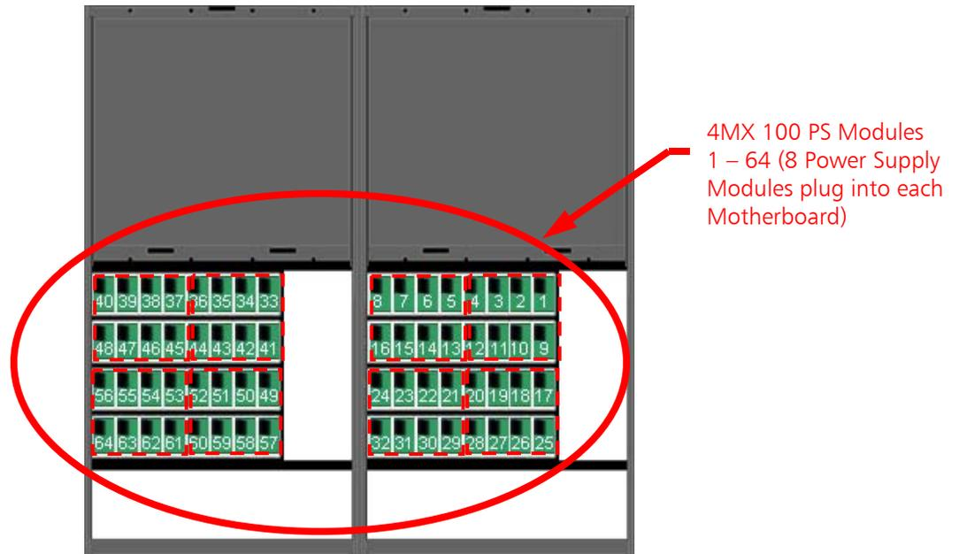
**Figure 145 – 4MX 100 Power Supply Module Locations (Rear of Transmitter)**
