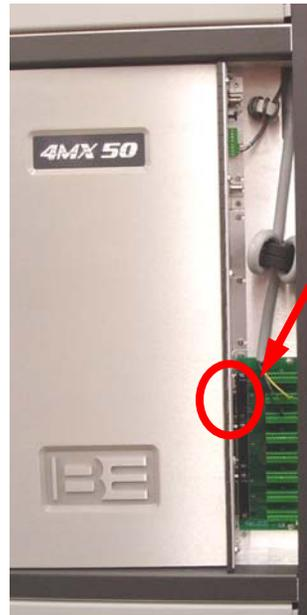
**Figure 180 – Remote Control I/O Access Panel Removal**
