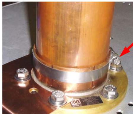
**Figure 27 – 4-1/16 Inch, 50 Ohm, RF Output Connection**
