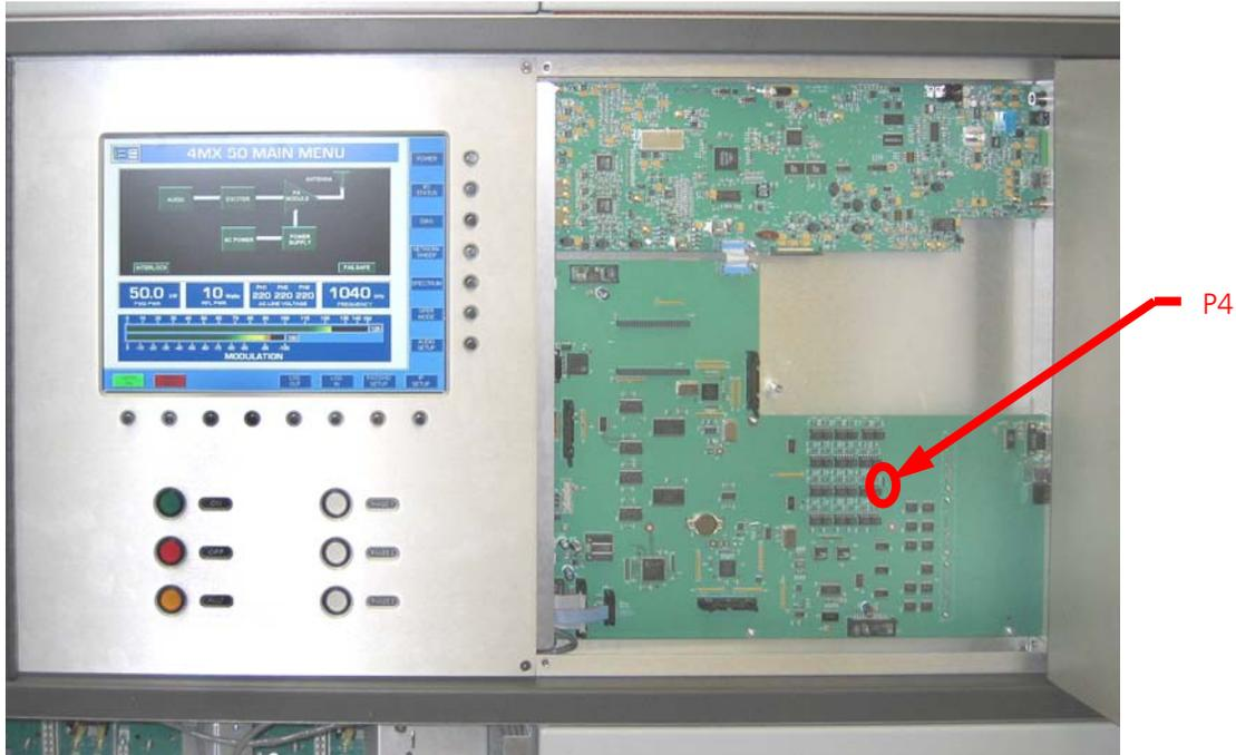
**Figure 40 – Controller Board I/O Signal Configuration Jumper**
