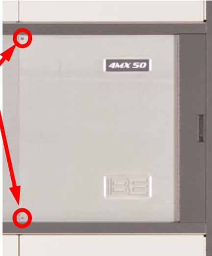
**Step 6b** – Using a No. 2 Phillips Screw Driver remove the (3) screws from the hinge area as shown
