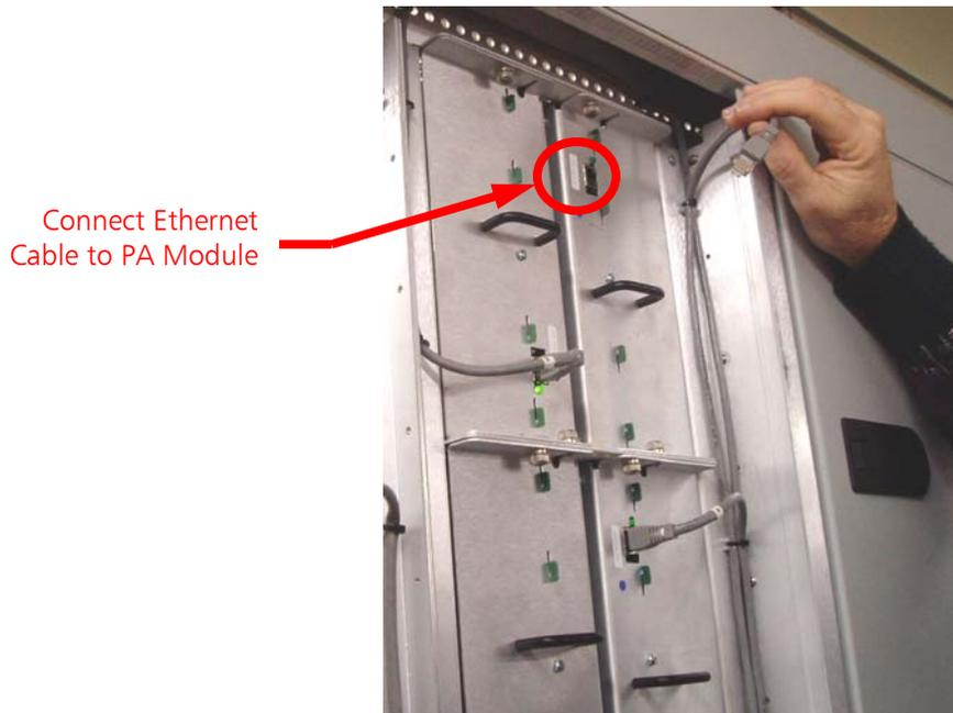
**Figure 105 – Connect the Ethernet Cable To PA Module**
