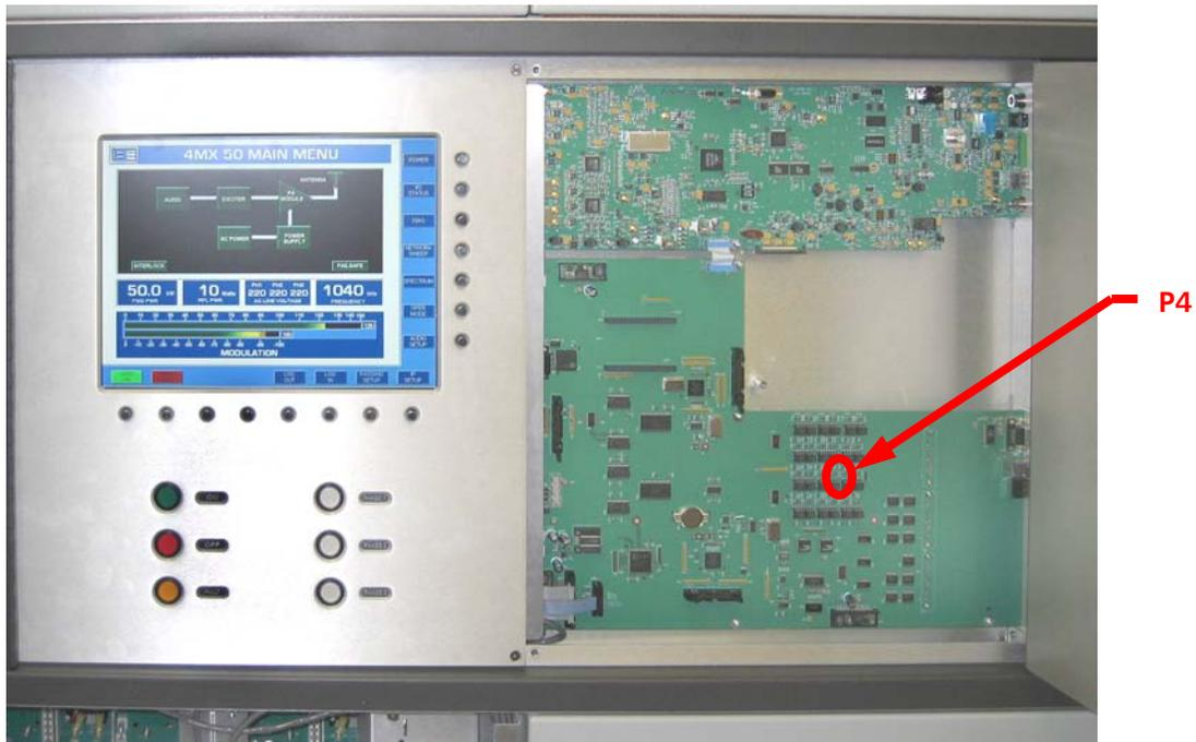
**Figure 89 – Controller Board I/O Signal Configuration Jumper**
