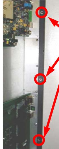
**Step 3** – Use the fold-out handle to remove the Remote Control I/O and Audio Input Access Panel
