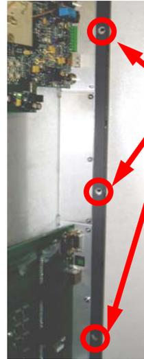
**Step 6c** – Use the fold-out handle to remove the Remote Control I/O and Audio Input Access Panel
