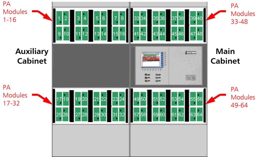
Figure 2 – 4MX 100 Front View (PA Module Locations)
