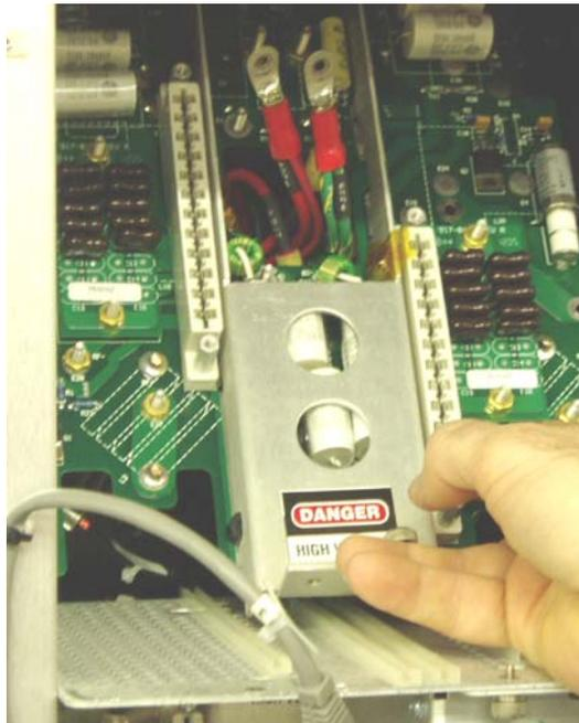
**STEP 2** – Once the coils clear the screw bosses, tilt the Motherboard to vertical position.
