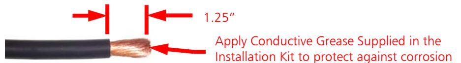
**Figure 34 – Suggested Strip Length and Grease for AC Supply Wiring**
