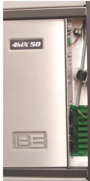
Figure 157 – Remote Control I/O Access Panel Removal
