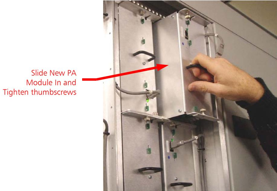
**Figure 104 – Install New PA Module and Tighten Thumbscrews**
