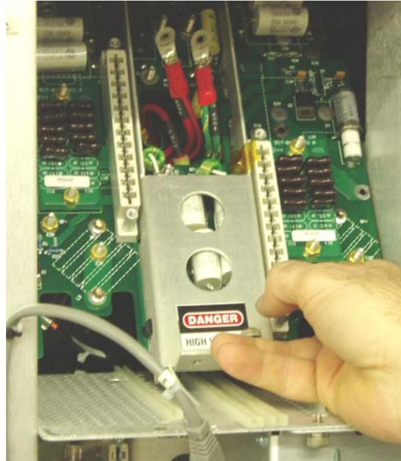
**STEP 2** – Tilt the Motherboard to horizontal position
