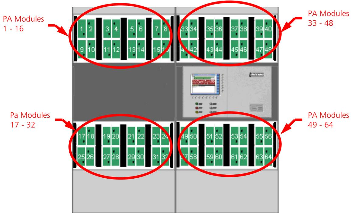
**Figure 100 – 4MX 100 PA Module Locations (Front of Transmitter)**
