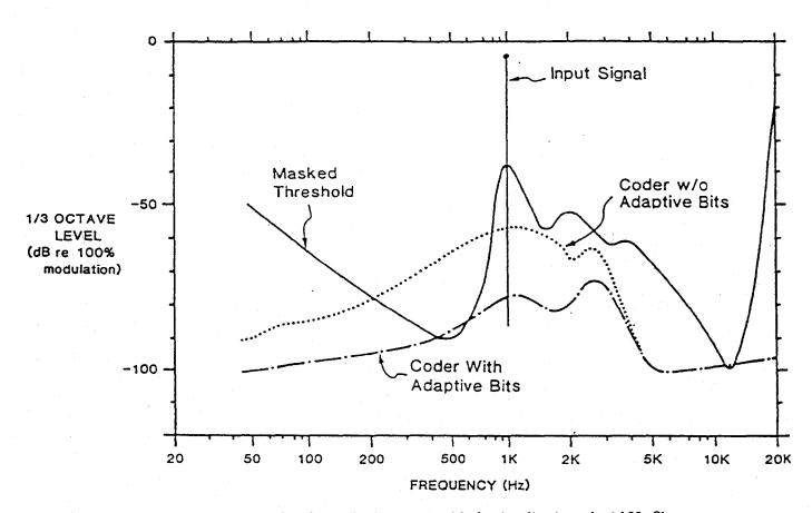
Fig. 6 Low Time Delay AC-2 Coder Performance with the Application of a 1 kHz Sinewave
