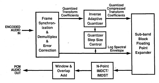
Fig. 8 AC-2 Digital Audio Decoder Family Block
