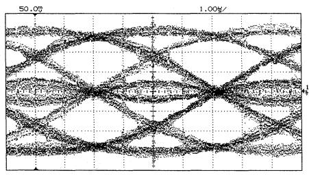
Fig. 9.11 Appearance of normal I or Q data pattern during test mode
