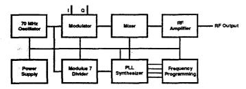
Fig. 4 DSTL Exciter Module Block Diagram
