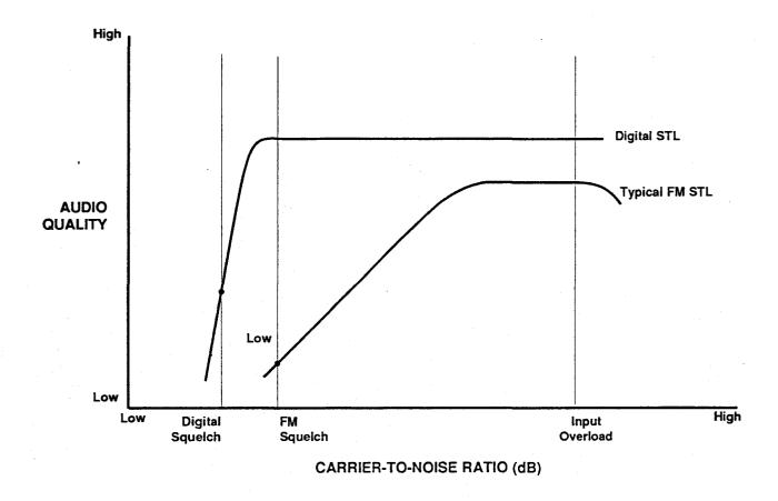
Figure 1: RF Carrier to Noise Ratio vs. Audio Quality Comparison for Typical FM and Digital Studio to Transmitter Links.
