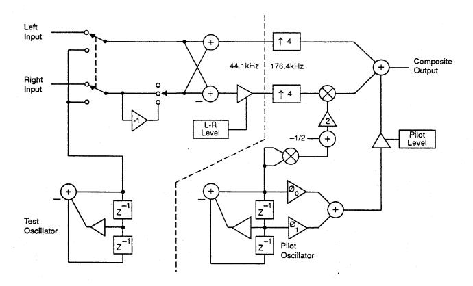
Figure 4. DSP Algorithm for Digital Stereo Generator
