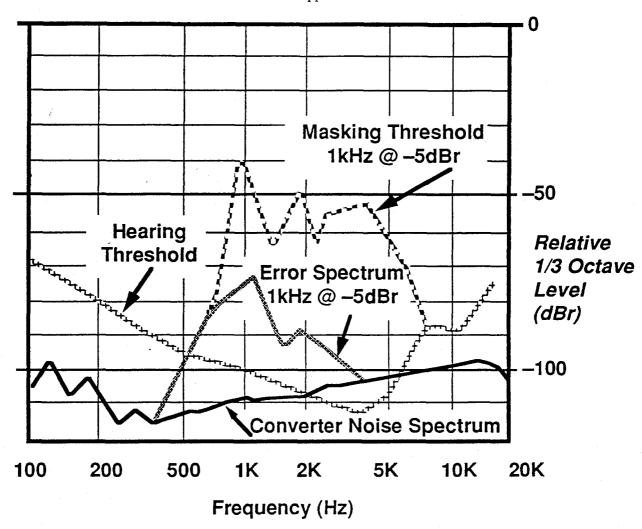
Figure 6: ADC + DDAC + AC-2 Coder Noise Spectrum for 1kHz Tone Compared to Masking Threshold.
