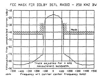
Fig. 8 Occupied Spectrum Mask of DSTL
