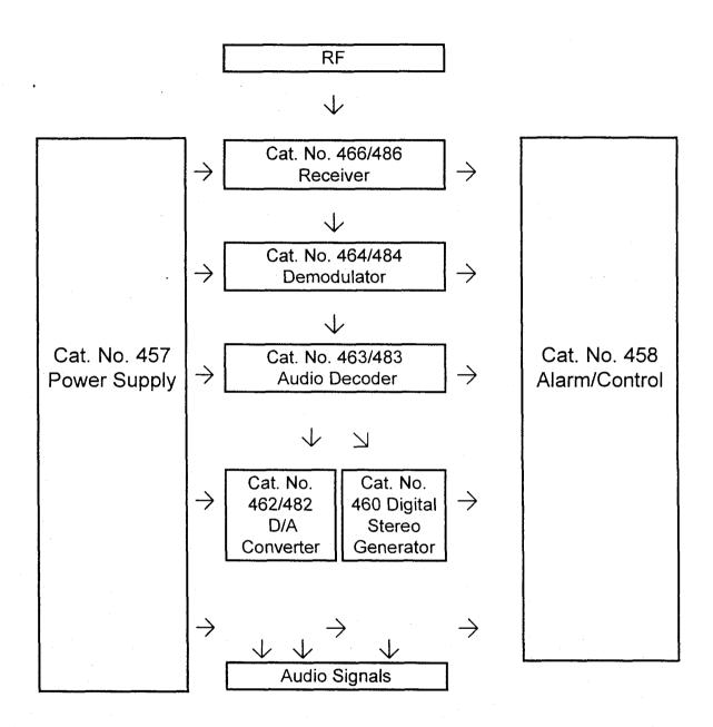
Fig. 9.4 Signal Flow, DSTL Receiver
