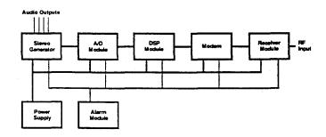
Fig. 9 Receiver Block Diagram
