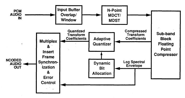
Fig. 7 AC-2 Digital Audio Encoder Family Block Diagram
