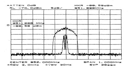
Fig. 8.5 Co-channel interference from an analog STL
