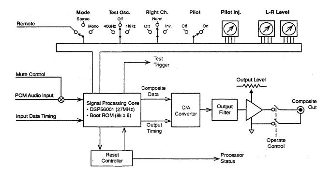
Figure 3. Stereo Generator Functional Block Diagram
