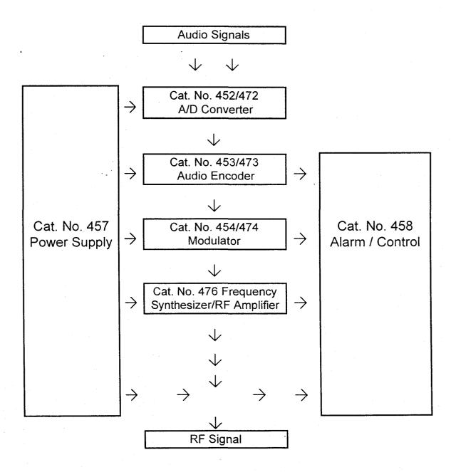
Fig. 9.3 Signal Flow, DSTL Transmitter
