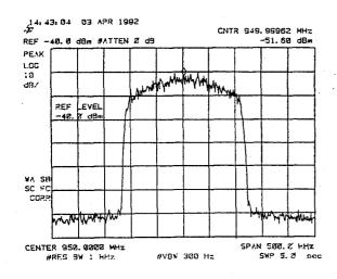
Fig. 8.2 Typical DP5501A transmit spectrum
