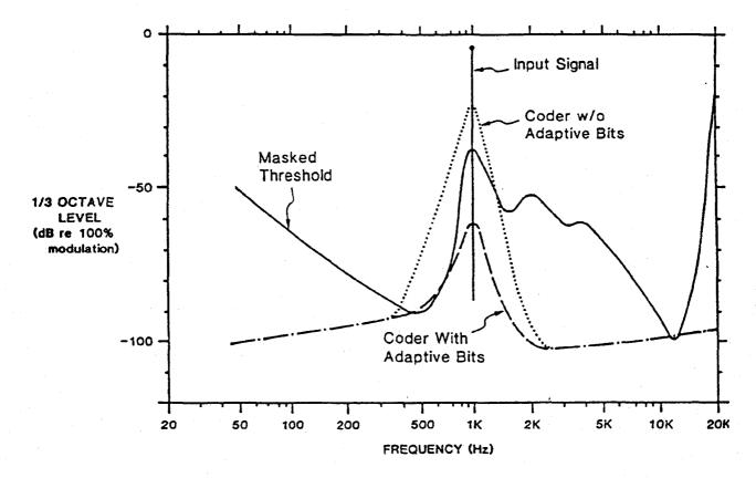
Fig. 5 Moderate Time Delay AC-2 Coder Performance with the Application of a 1 kHz Sinewave
