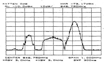
Fig. 8.4 Receive spectrum in the presence of adjacent channel STLs
