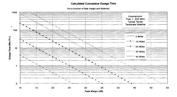
Figure 1 Typical Outage Time Nomograph
