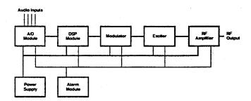
Fig. 3 DSTL Transmitter Block Diagram.
