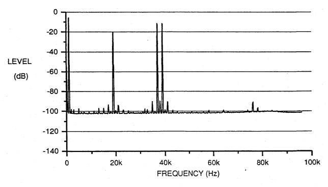
Figure 6. Spectrum of Composite Analog Output for Left Channel Modulation
