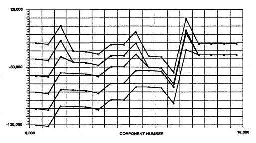
Fig. 12 AGC Budget Analysis for Various Input Levels
