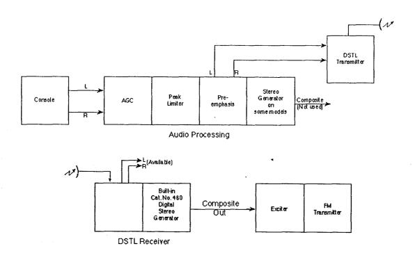
Fig. 2.1 DSTL with internal digital stereo generator creates a "virtual composite" link
