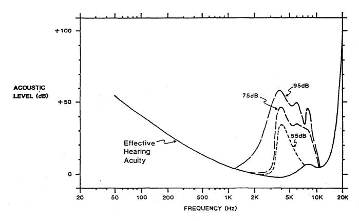
Fig. 3 4 kHz Masked Threshold Curves (0 dB = 20 micropascals)
