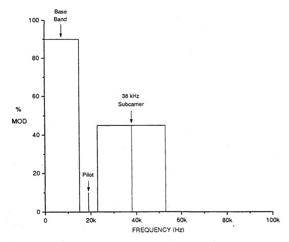
Figure 2. Composite Stereo Signal Spectrum
