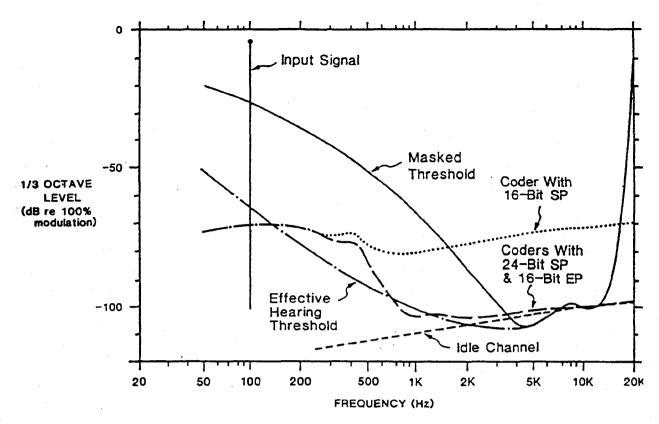
Fig. 9 Comparison of Filter Bank Arithmetic Noise of Single Precision (SP) 16-bit Arithmetic Versus Extended Precision (EP) 16-bit and Single Precision 24-bit Arithmetic
