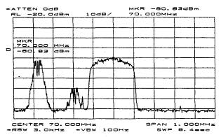
Fig. 8.6 Adjacent channel analog STL interference
