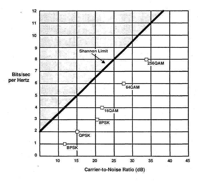
Figure 4: Spectral Efficiency vs. Carrier-to-Noise Ratio for Various Digital Modulation Schemes.
