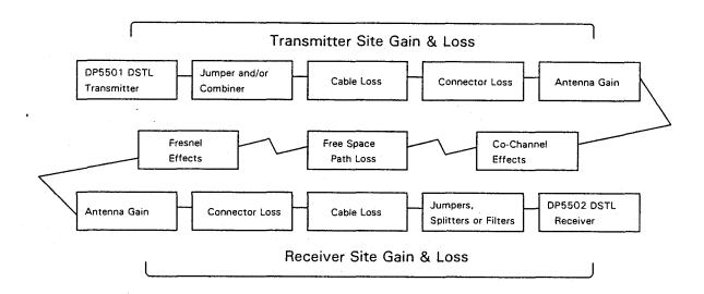
Figure 2 DSTL system block diagram for path loss calculations.
