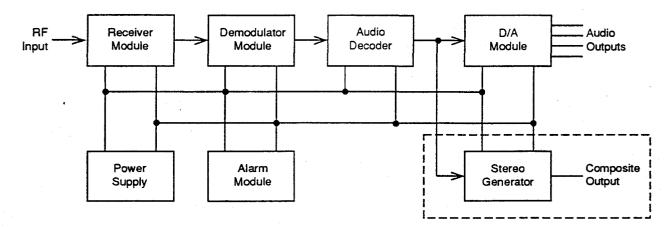
Figure 1. DSTL Receiver Block Diagram
