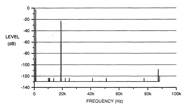
Figure 7. Spectrum of Composite Digital Output for Left + Right Channel Modulation
