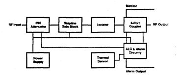
Fig. 5 DSTL Power Amplifier Module Block Diagram
