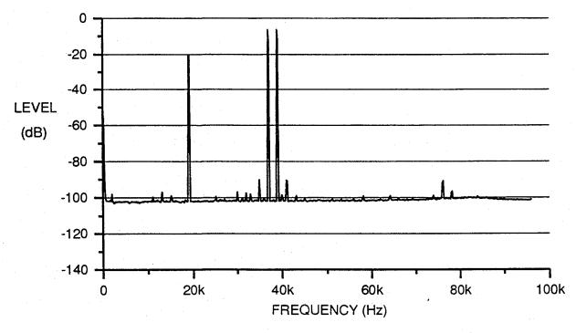
Figure 10. Spectrum of Composite Analog Output for Left – Right Channel Modulation
