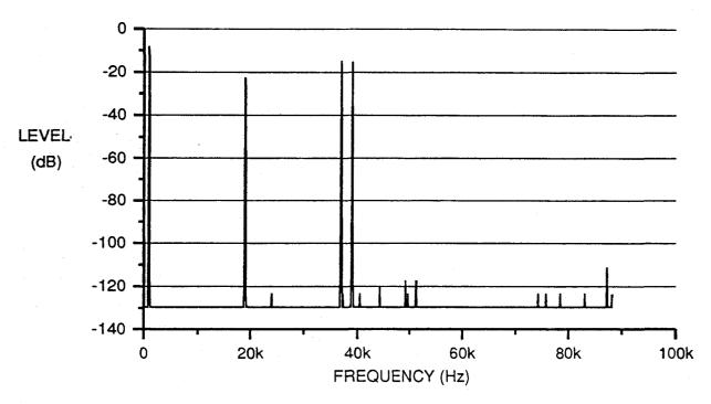
Figure 5. Spectrum of Composite Digital Output for Left Channel Modulation
