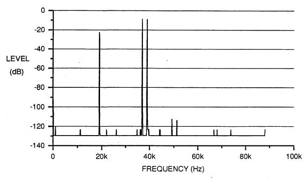
Figure 9. Spectrum of Composite Digital Output for Left – Right Channel Modulation
