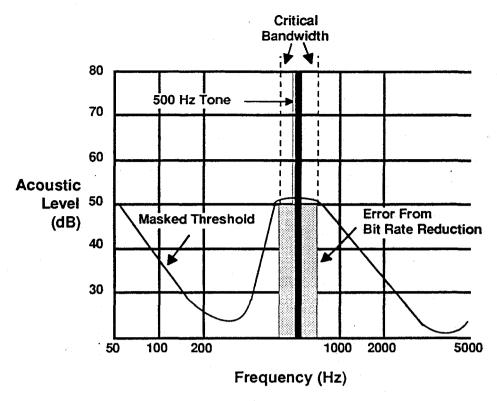
Figure 5: Comparison of Critical Band Masking and Optimal Coder Performance for a 500 Hz Sinewave Signal.
