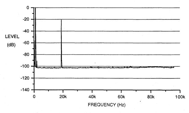
Figure 8. Spectrum of Composite Analog Output for Left + Right Channel Modulation
