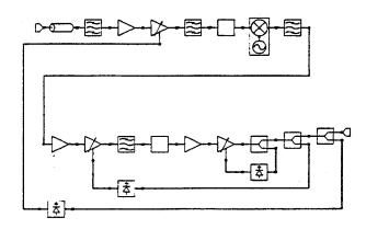
Fig. 11 DSTL Receiver AGC Block Diagram
