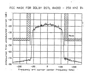
Fig. 8.3 Typical DP5501A transmit spectrum with mask applied
