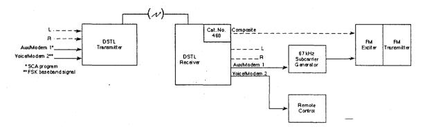
Fig. 2.2 Typical usage of Aux and Voice channels with DP5501A/5502
