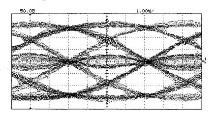
Fig. 8.1 Typical eye pattern in TEST mode
