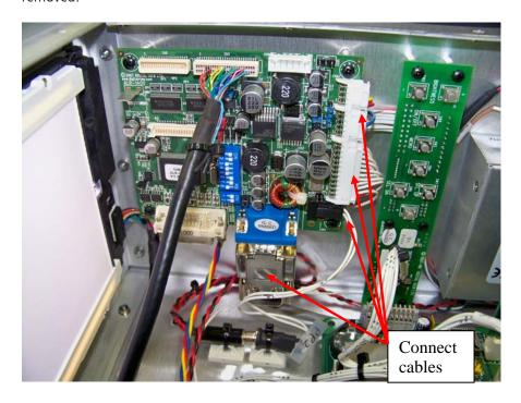
5. Install power adapter cable to existing power cable and ATR-1400 video cable:
