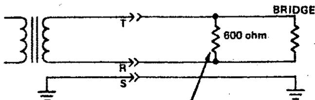
TERMINATION RESISTOR ADDED TO PROPERLY LOAD UNIT
