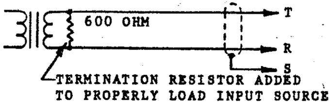
UNBALANCED LINE FROM 600 OHM TRANSFORMER
