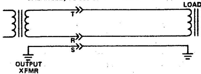
**UNBALANCED, TO 600 OHM TRANSFORMER**
