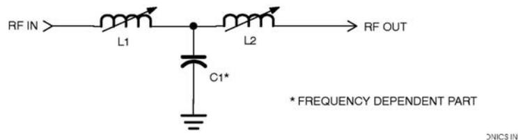
Figure 1 – SCHEMATIC - AM MATCHING NETWORK
