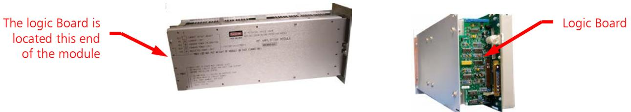
**Figure 43 – RF Amplifier Module Logic Board Location**
