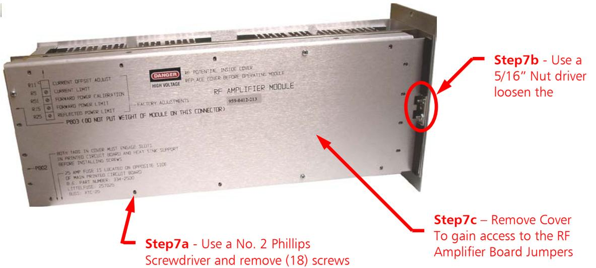
Figure 46 – RF Amplifier Module Cover Removal
