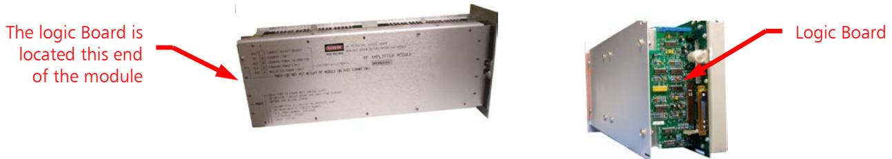
**Figure 5 – RF Amplifier Module Logic Board Location**
