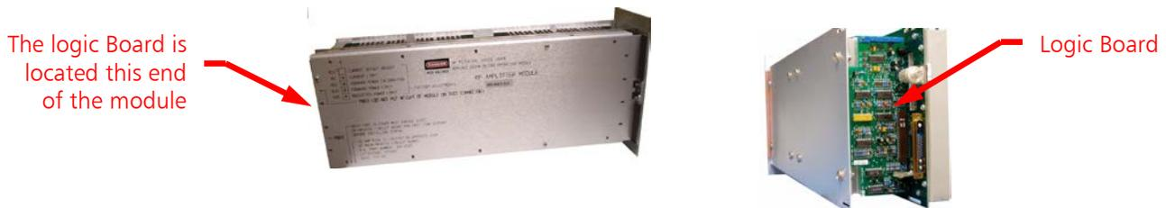
**Figure 27 – RF Amplifier Module Logic Board Location**
