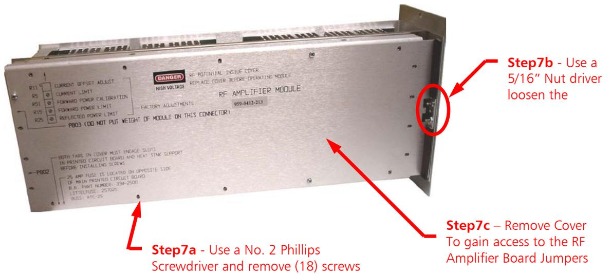
Figure 30 – RF Amplifier Module Cover Removal
