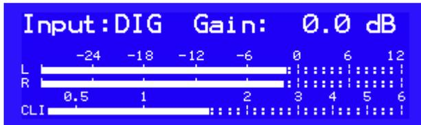
The bars are showing the input signal peak level: the input level must be adjusted to have the reading peaking around 0dB. The single bar below shows, with a long decay time constant, the instantaneous clipping level of the input signal. Short peaks up to +3dB are quite normal, especially when the input signal, despite it was already compressed - limited by a suitable FM broadcasting processor, is then transferred through MPEG compression.
