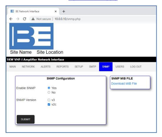
The SNMP page also allows for the SNMP service to be enabled and disabled. The user may also select between SNMP v2c and the more secure SNMP v3. Please not the user account created under the Users page will be used to access SNMP v3. The password requirement for SNMP is a minimum of 8 characters.
