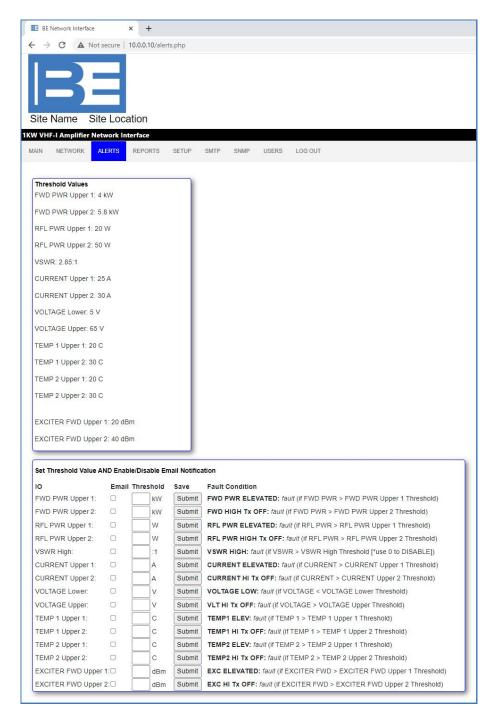
Descriptions to the right of the input boxes provide details of the fault displayed and the condition that causes it to occur. Faults are available on the Ethernet network interface (GUI and SNMP), and the DB9 Remote Connection.
