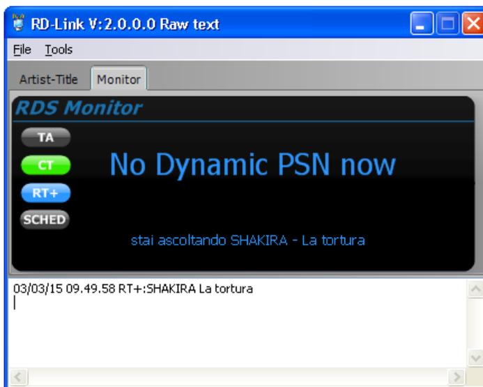
On the **Monitor** window the dynamic PS and Radiotext strings are shown in the same way as they are being transmitted.
