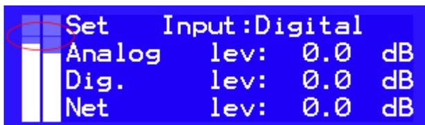
The initial adjustment of the input level should be made so that the maximum analog input level is equal to or only slightly above that limit.
