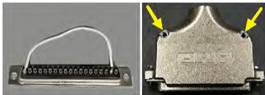
GPIO Failsafe Jumper, (see Technical Manual 2.2.7, Figure 13)
